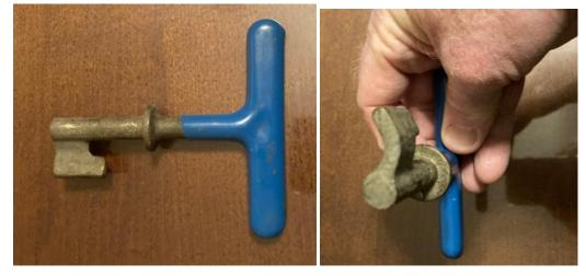
You remove the water valve cover by inserting the tool into the keyhole in the cover as shown in photo below. You remove the cover by turning the tool counter-clockwise and lift the cover with the tool inserted. It may take a little manuevering to get the cover off.
